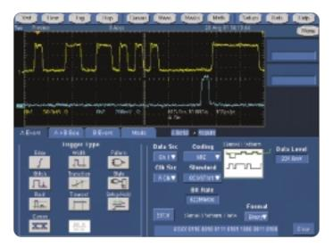
Figure 9. CSA7000 Series serial pattern trigger menu.
