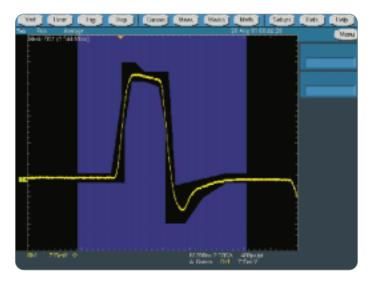
Figure 8. A DS1 mask where the leading and trailing bits surrounding the logic one pulse must be zero for at least one bit time. The signal shown is known as an isolated one.
