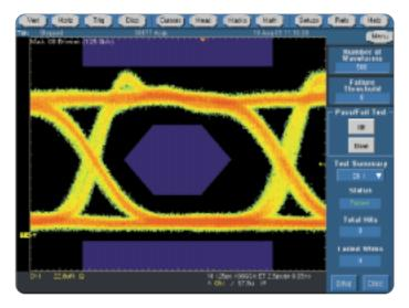
Figure 5. Gigabit ethernet eye diagram with the optical reference receiver filter turned off.
