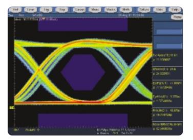
**Figure 10.** Intensity-graded eye crossing display.
