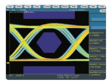
Figure 6. Verifying compliance with a communications standard requires several tests such as pulse width, amplitude, extinction ratio, Qfactor, eye height and width, noise and jitter measurements. Using a DPO, many of these tests can be performed in the development lab, in manufacturing or on-site at a network installation.
